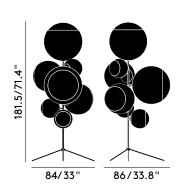
A steel fabricated stand with vacuum metallised shades. The process involves vaporising a small amount of pure metal at a very high temperature and then sucking it onto a surface by applying an electrical charge.
